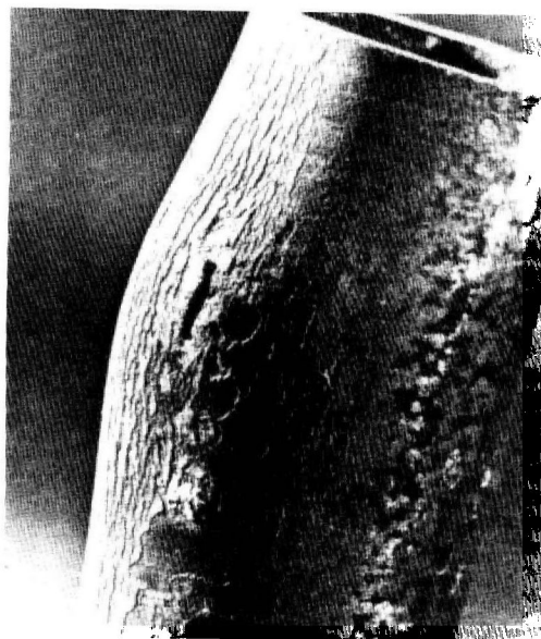
Figure 1-5. Tube Blister Due to Periodic Overheating Note fissure and creep cracks, typical result of alternating overheating and cooling.
