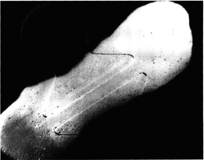
Fig. 4 The first metal-oxide-semiconductor field-effect transistor. 13 (Photograph courtesy of Bell Laboratories.)
