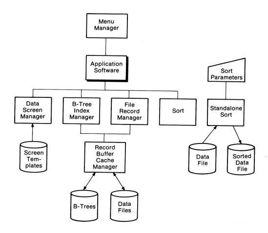
Figure 1-1. C tool functions: system architecture.
