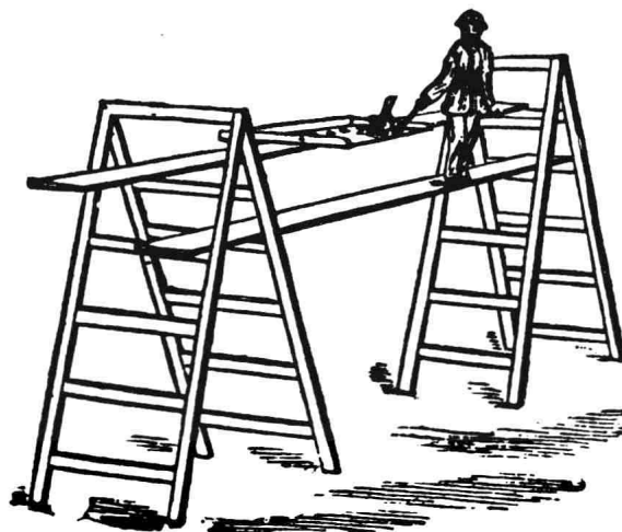
Flying horses, F. Lloyds's suggested alternative to the flying bridge ( Practical Guide to Scene Painting and Painting in Distemper )
