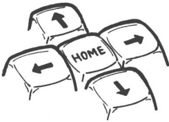
Fig. 1.5 Special function keys are often added to the standard typewriter keyboard for moving the cursor up, down, left, or right on the screen. The "home" key would usually be programmed to move the cursor directly to the upper left-hand corner of the screen. Some systems may have ten or more special function keys for cursor movement and other operations that are specific to word processing.
