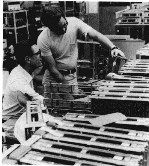
Hewlett-Packard engineers ponder changes in a circuit board and its supporting structure, an essential module of the professional oscilloscopes shown in the foreground. Engineers are always alert to changes that will improve equipment performance and reliability. (Photo courtesy of Hewlett-Packard)
