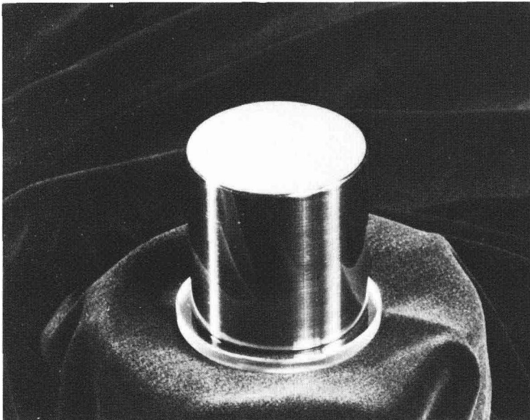
Fig. 1-2. Prototype kilogram 20, the mass standard in the custody of the National Bureau of Standards. It is an exact duplicate of the mass kept by the Internal Bureau of Standards at Sèvres, France. (Courtesy National Bureau of Standards.)
