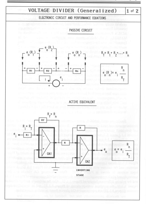
Figure 1.1.1 The generalized voltage divider.
