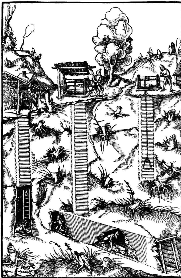
FIG. 1.3. First stages in the excavation of a mine (from Agri-cola, De Re Metallica , 1556).
