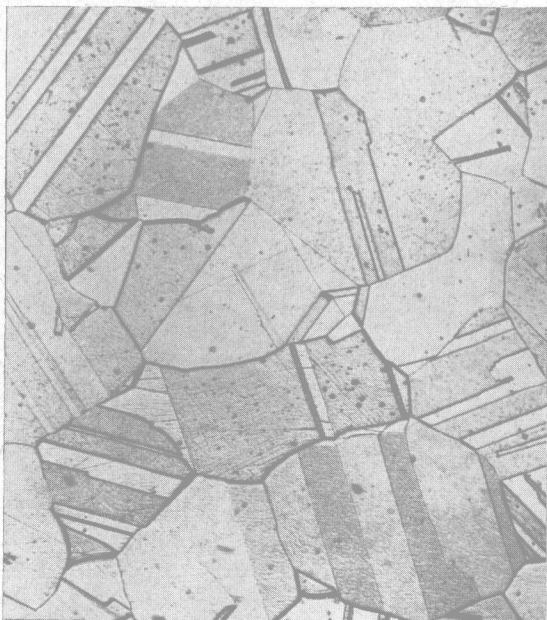
FIG. 1.3. Illustration of grain structure in a recrystallised 70/30 brass ( \times 100 ).
