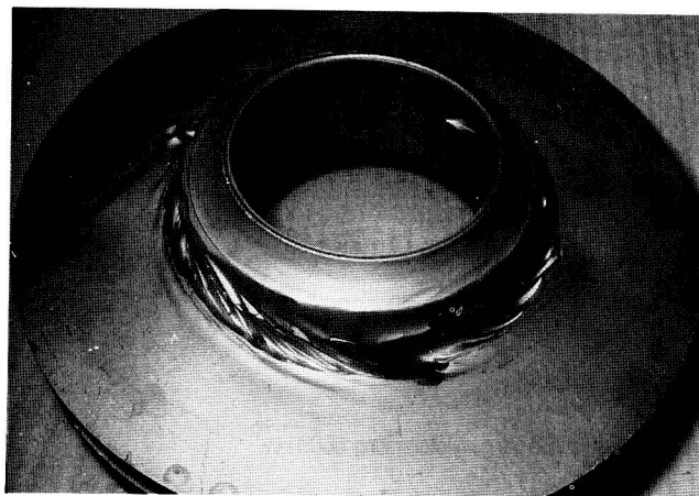
Fig 8 Duplex stainless steel impeller after 6 months in produced water service
