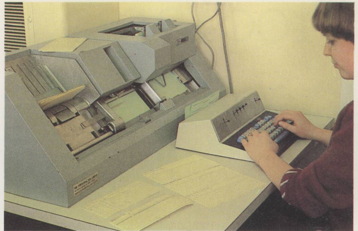
This keypunch operator is typing letters and numbers on the keyboard. The machine converts the letters and numbers into holes it punches in the cards.
