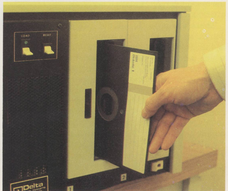
An increasingly popular form of input is the floppy disk, here shown being inserted into the disk drive of a small computer system. This disk can hold 576,000 characters of data, others can hold as many as 1,100,000 characters.
