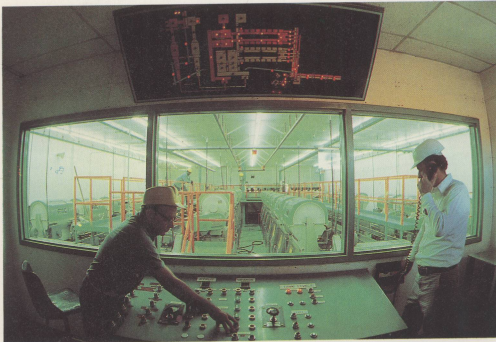
The panel of a computer that is used to control the production of orange juice. It indicates the levels of the juice in the tanks and controls the extraction process. The lighted panel above the window shows the flow of juice throughout the factory.
