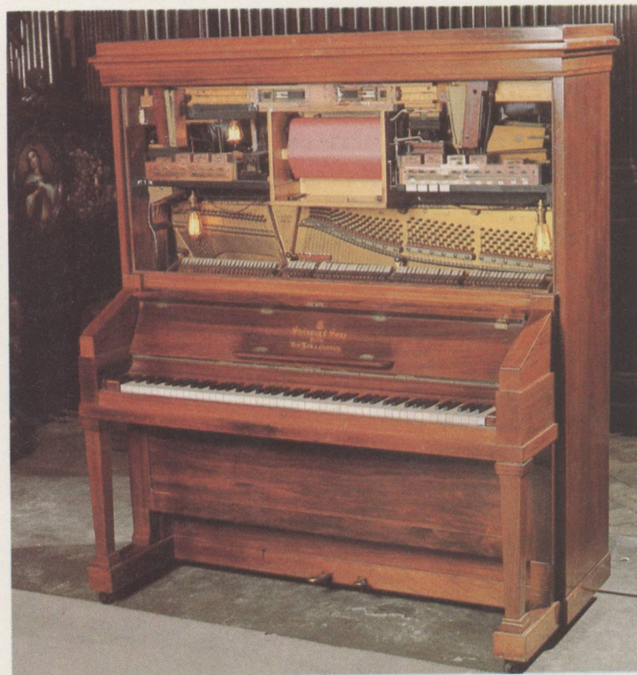
In this upright Steinway player piano, made in 1910, the roll of programmed paper can be seen in the center in pink. The player piano was patented in 1879 by E. H. Leveaux of Surrey, England.
