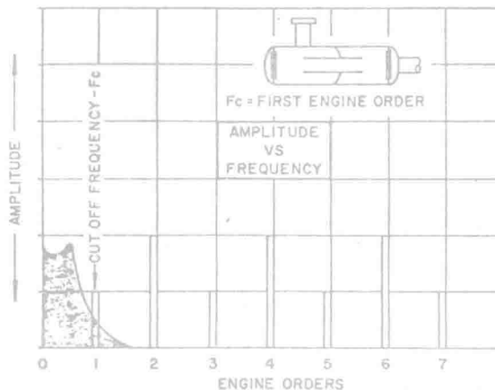
Fig. 4. Acoustical response when cut-off frequency equals the first engine order.
