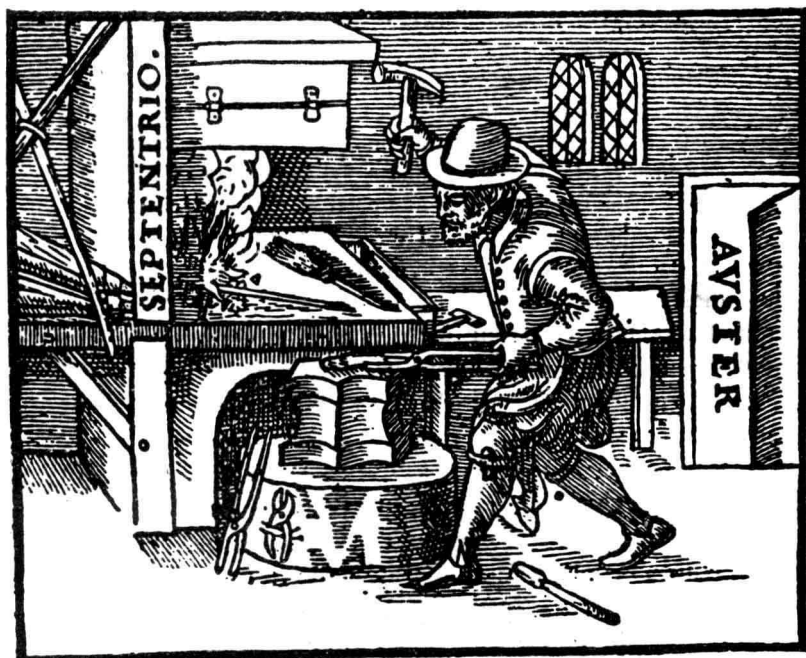
Figure 1-3. Smoothing an iron rod in the direction of the Earth's field, as shown in Gilbert's De Magnete . (Septentrio, north; auster, south.)
