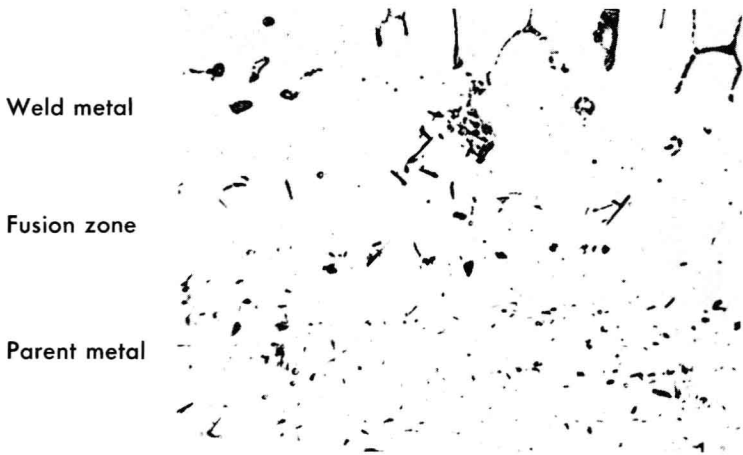
Interface at weld and parent metal for argon-shielded tungsten-arc weld in 1100 alloy with 1100 filler metal.
