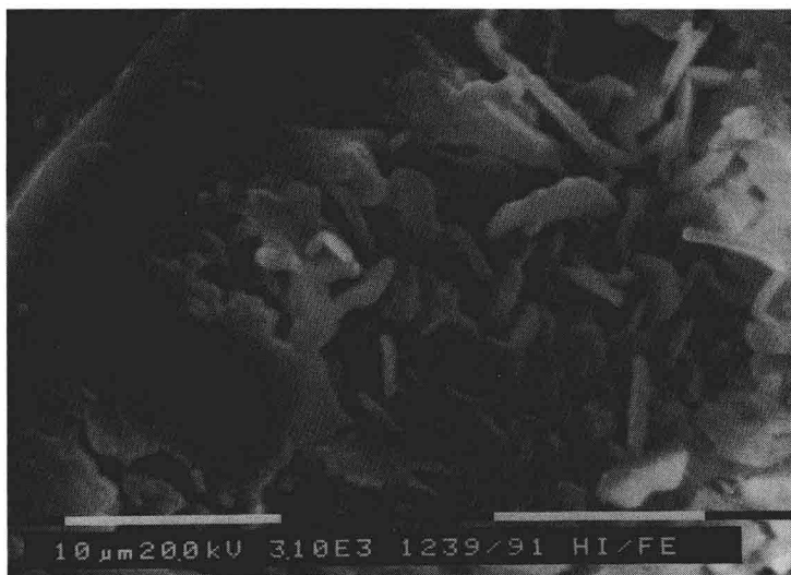
Figure 1.2 Cross-section of polypropylene prepolymer. Polymer : catalyst ratio 1:1 (wt%) ( \times 3100 ).
