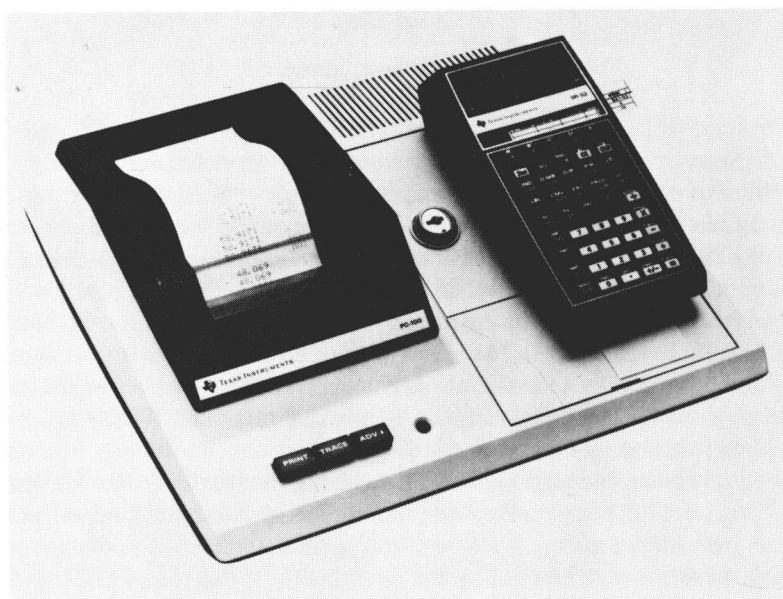
Fig. 1.3 Texas Instruments PC 1000 printer cradle with an SR 52 in place.
