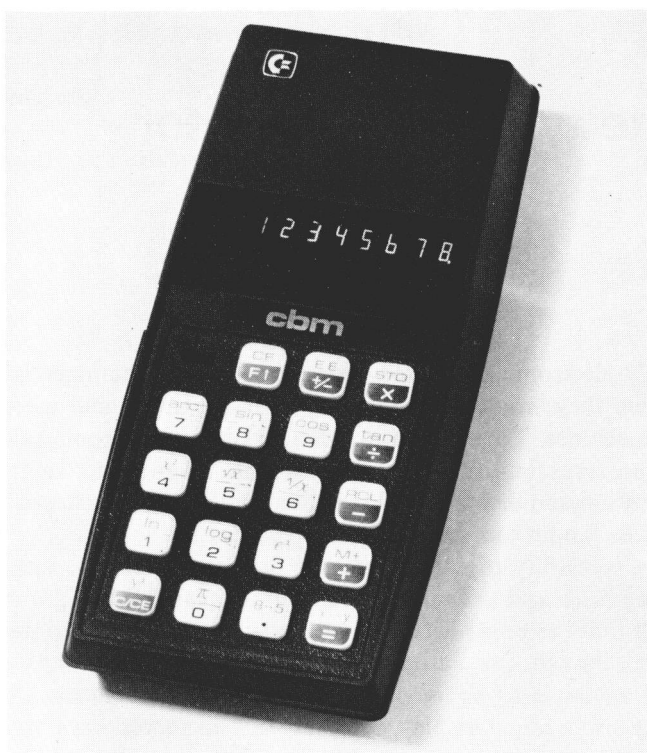
Fig. 1.1 Example of a 'semi-scientific' calculator.
