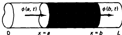
Figure 1.2.2 Heat energy flowing into and out of a finite segment of a rod.
