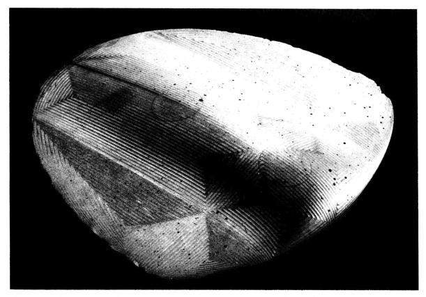
Figure 1.1 A premiere model from 1962: the 'Flying Saucer'. Notice the spiral machining marks and the rectangular and triangular patches.
