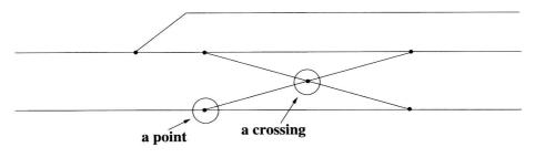
A point is a device allowing a track to split in two distinct directions. A crossing, as its name indicates, is a device that makes two different tracks crossing each other. In what follows we briefly describe points and crossings.
