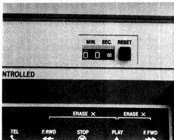
Illus. 1-4 Counter Wheel, Often Used with an Index Log
