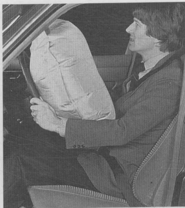
New fibre technologies and safety: this electronically triggered airbag, developed by Mercedes-Benz, inflates within thirty milliseconds in the event of a car crash.
