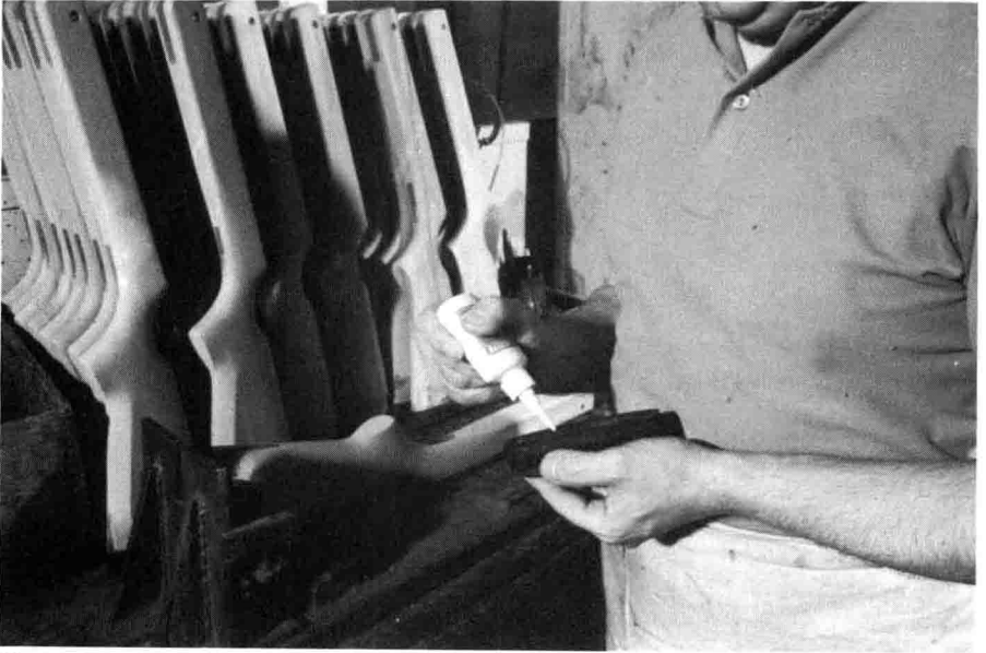
Figure 1.4 Fast, room-temperature hardening, single-part cyanoacrylate adhesives are widely used for bonding metallic, plastic, rubber and wooden substrates, such as in attaching the rubber recoil pad to this hardwood gun stock.
