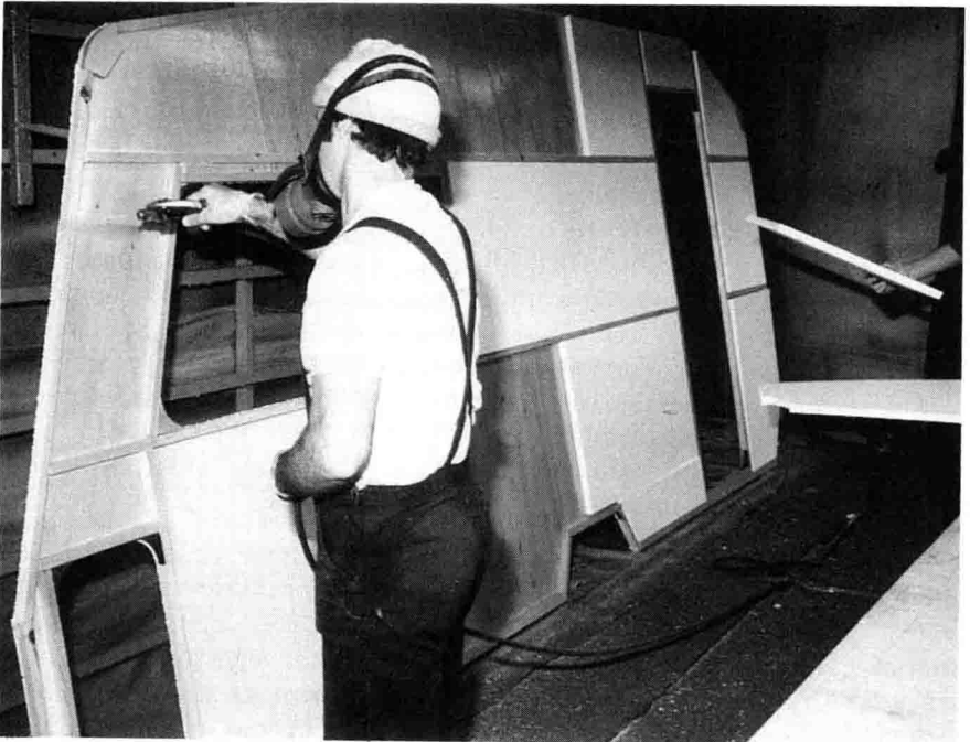
Figure 1.1 A caravan sandwich panel being sprayed with a moisture-hardening rubbery polyurethane adhesive, in a solvent, prior to bonding on the inner skin. The absence of mechanical fasteners greatly increases the production rate and results in a more pleasing appearance.
