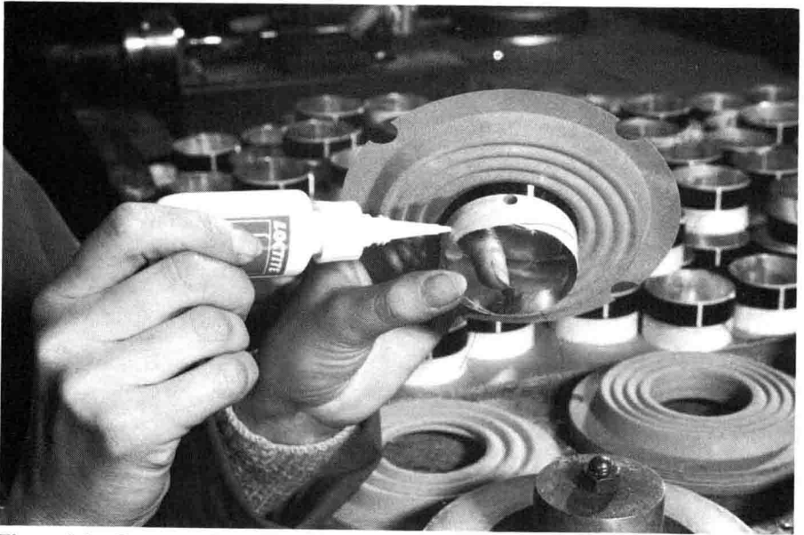
Figure 1.5 Cyanoacrylate adhesives are also used to assemble loudspeakers.
