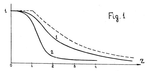
wave fluctuations are strongly smoothed. On fig.1 intensity damping for the harmonic signal (dotted line) is also shown. The comparison shows that transmission of regular signal at large distances is more advantageous energetically.
