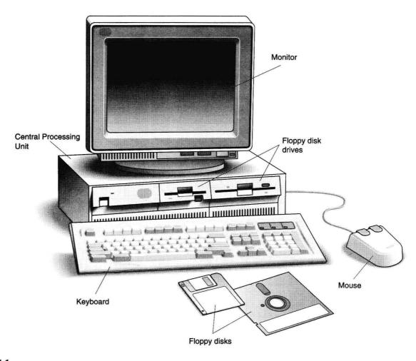
FIGURE 1.1 \_\_\_\_ Microcomputer Hardware Components
