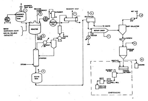
FIGURE 2: SIMPLIFIED FLOW DIAGRAM FOR BATCH EMULSION POLYMERIZATION OF VINYL CHLORIDE
