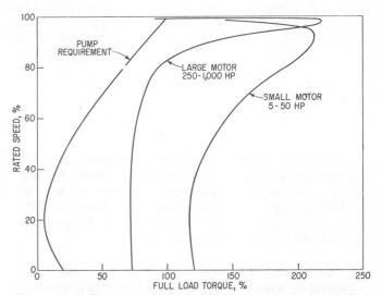
Figure 1-8. Typically large motors have relatively smaller capacities for accelerating their loads than small motors. Special designs can lessen the difference, but seldom eliminate it.
