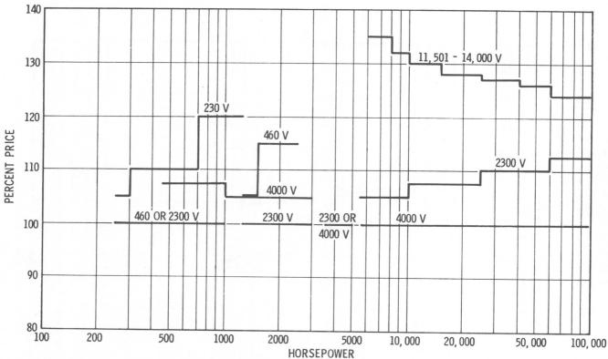
Figure 1-5. Cost vs. voltage for synchronous motors. Percentages refer to base prices shown in Figures 1-2 and 1-3. Read from left to right; at steps use first value reached.
