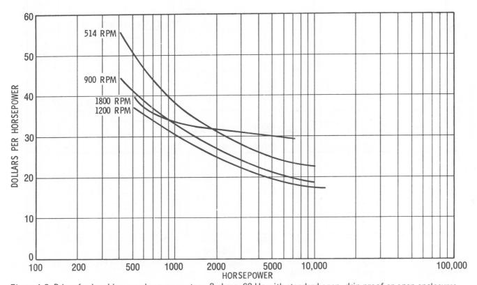
Figure 1-3. Prices for brushless synchronous motors, 3-phase, 60 Hz with standard open, drip-proof or open enclosures.
