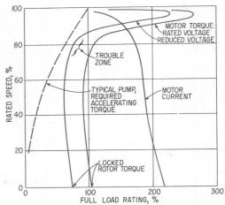
Figure 1-7. Startup difficulty probably occurs at the "trouble zone" in a typical, large 3,600-rpm motor accelerating a centrifugal pump.
