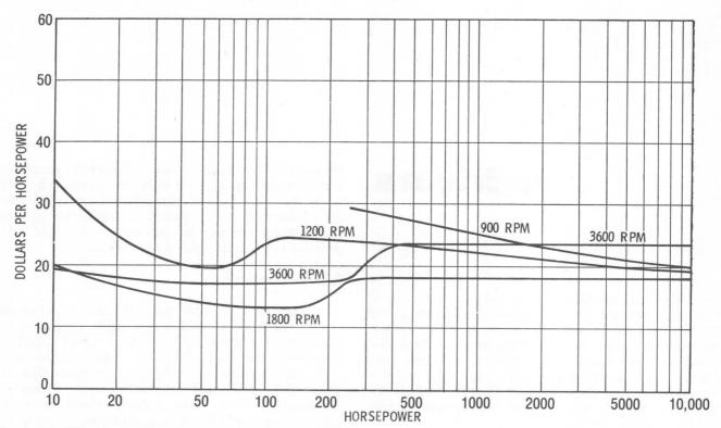
Figure 1-1. Prices for squirrel-cage induction motors, 3-phase, 60 Hz with standard voltages and open, drip-proof enclosures.
