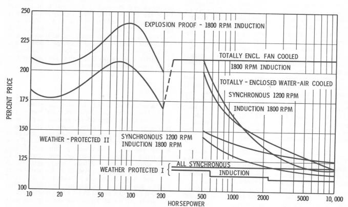
Figure 1-6. Approximate percentage price vs. various enclosures for induction and synchronous motors. Curve applies to Figures 1-1, 1-2 and 1-3 after application of Figures 1-4 and 1-5.
