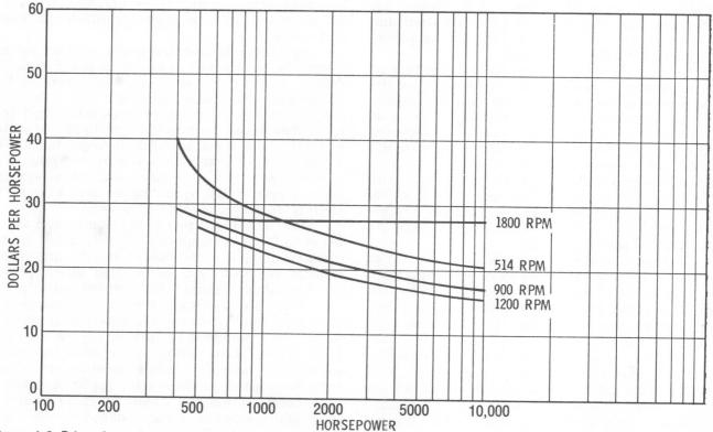
Figure 1-2. Prices for conventional synchronous motors (with slip rings), 3-phase, 60 Hz with standard voltages and open, drip-proof enclosures.
