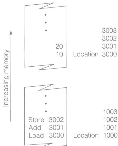
Figure 1.4 Representation of machine-language program and data stored in computer memory
