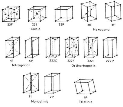
Figure 1. Fourteen Bravais lattices: letters P, F, I, and C represent type of lattice; numbers represent the symmetry axes.
