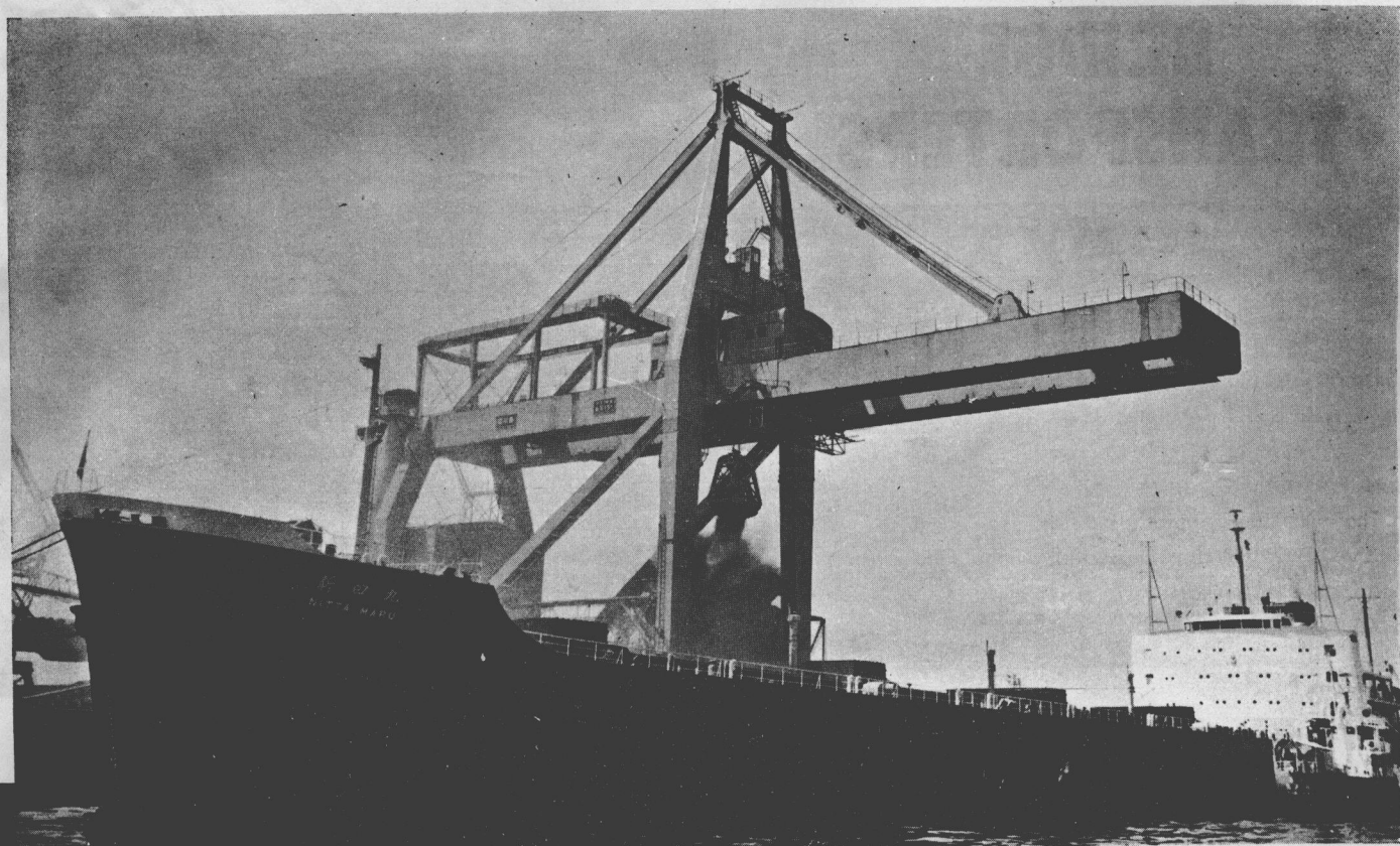
Fig. 3 帶有旋轉小車的每小時 1000 噸鐵礦與煤卸料機 1,000 t/h Ore and Coal Unloader with Turn-Table Man-trolley for Fuji Iron & Steel Co., Ltd.
