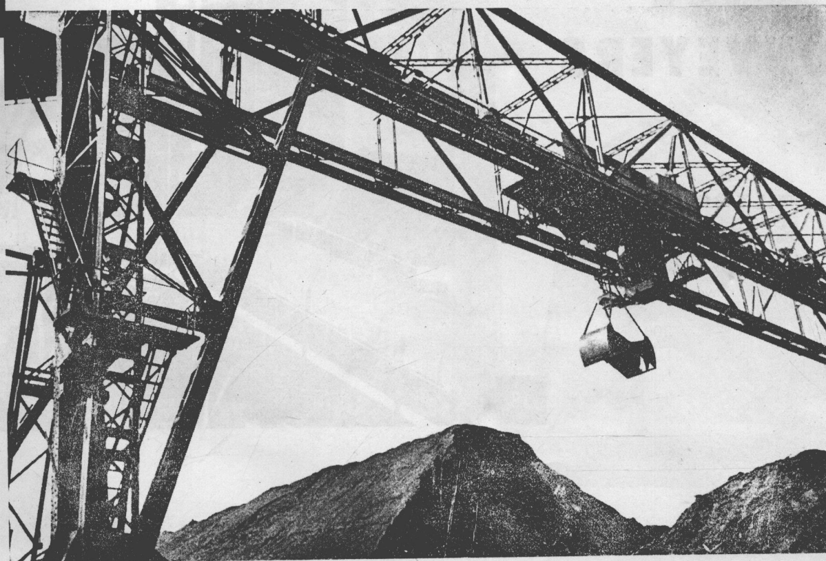
Fig. 16, 17 每小時 250 噸帶有小車的運載橋, 抓斗容量 5 噸 250 t/h Man-trolley Type Transporter with 5-ton Grab Bucket for Tokyo Electric Power Co., Ltd.
