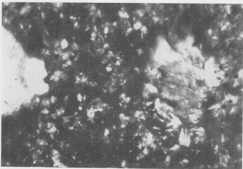
FIG. 1. Structure of molten Kahlenborn basalt. Microscopic picture of a thin section in transmitted polarized light. Magnification: 400\times
