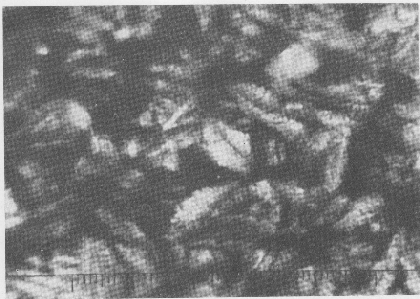
FIG. 3. Structure of molten Kahlenborn basalt. Picture of the same slide as in Fig. 1 in polarized light. Magnification: 1500\times , 1 division: 1\text{ }\mu\text{m}
