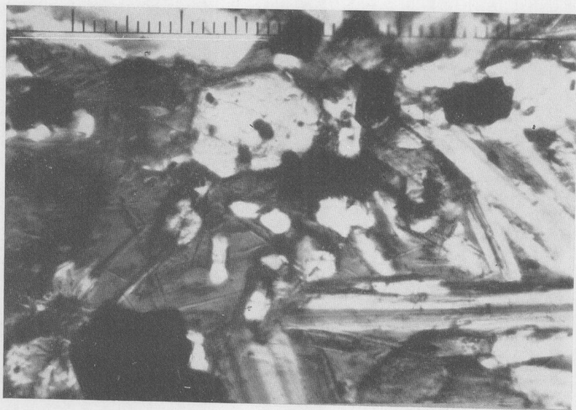
FIG. 5. Structure of Badacsony basalt. Microscopic picture of a thin section. Magnification: 400\times , 1 division: 5\text{ }\mu\text{m}
