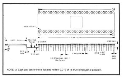
Fig. 2-1. The 64-pin dual inline package of the TMS9900 is larger than the more familiar 40-pin DIP configuration used by 8-bit microprocessors. Added 24 pins make possible more system interconnections. (Courtesy of Texas Instruments)
