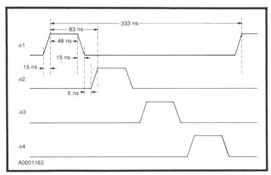
Fig. 2-2. Clock waveforms required by TMS9900 when operating at maximum 3-MHz frequency are shown here. Dead space of 5 ns between phases is essential to proper operation of processor. (Courtesy of Texas Instruments)
