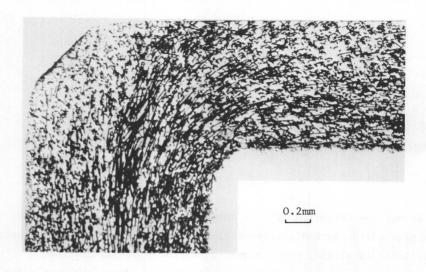
FIG. 2.1. Optical micrograph of a thin section taken from a carbon fibre reinforced nylon 66 moulding.
