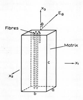
FIG. 2.2. Definition of axes used to describe mechanical anisotropy.
