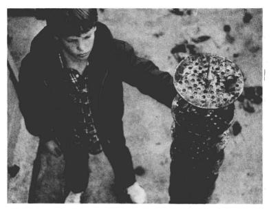
Fig. 1-4A. Stripper plates. Holes should be 13/32" in diameter and comprise 15 percent of the surface area of the plate.
