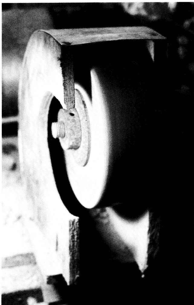
Felt polishing wheels. These are of two types: brown, coarse felt suitable for pumice and white felt which is now the most common type used for final polishing.
