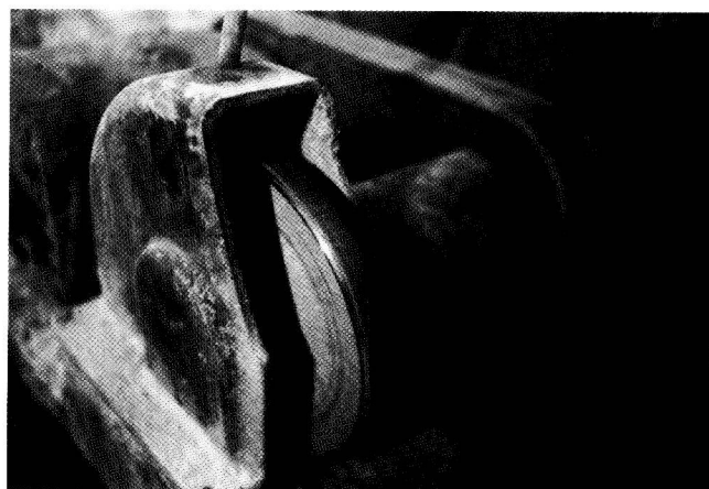
Coarse diamond wheel used for roughing out glass forms.
