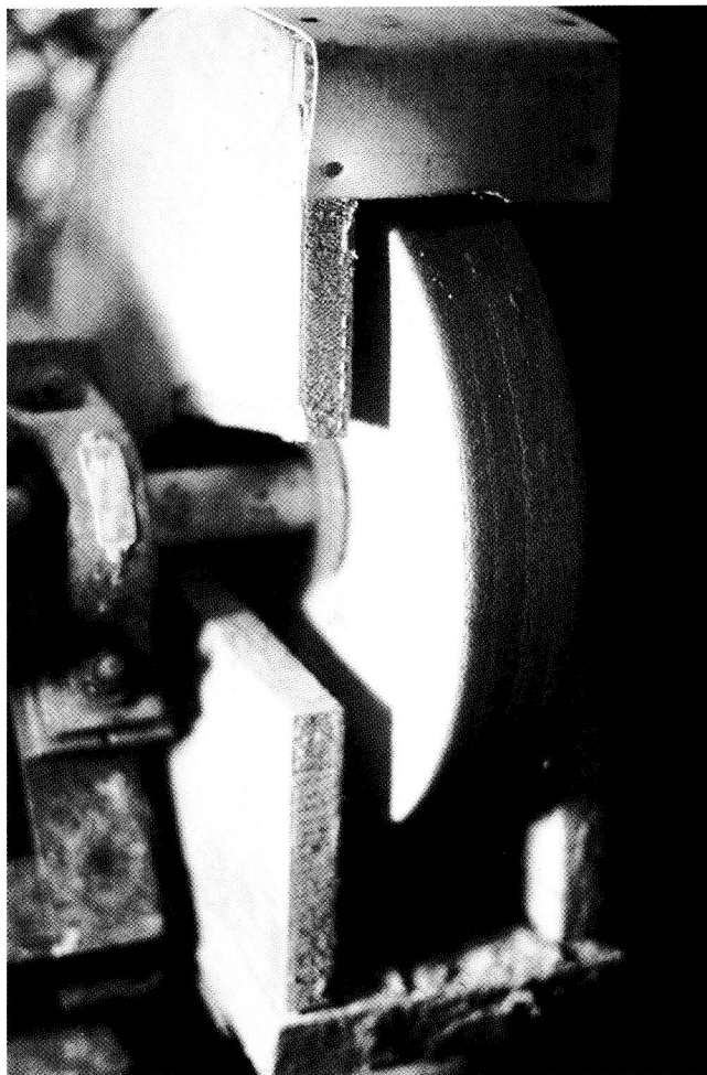
Composite fibre wheel currently the most popular for use with pumice.
