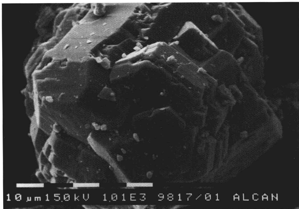
Figure 2. SEM of Gibbsite B as received.
