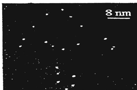
Fig. 8 The STM image of an umbrella-like recorded pattern on CPU monomer thin film 19 .
