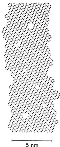
Fig. 1.2. Sketch of a typical graphene plane in a carbon fiber showing vacancy-cluster defects [Fourdeux et al. 1971]
