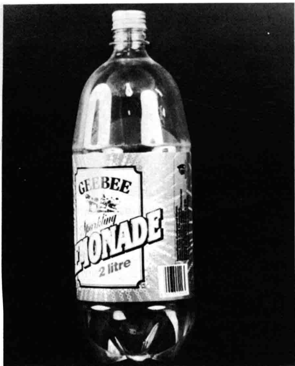
Injection blow moulded lemonade bottle in PET (polyethyleneterephthalate).
