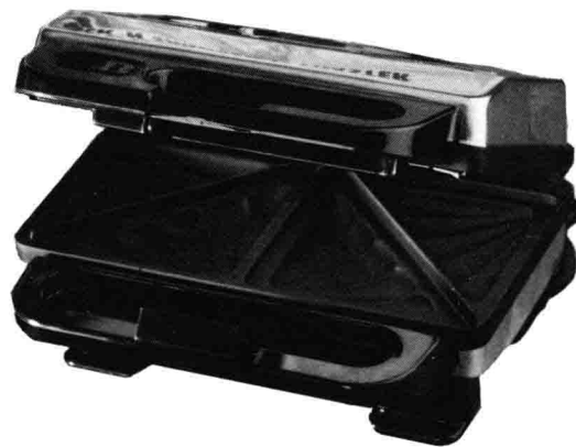
Sandwich toaster with phenol formaldehyde (bakelite) compression moulded, heat resistant handles and a non-stick coating of ptfе (polytetrafluoroethylene).
