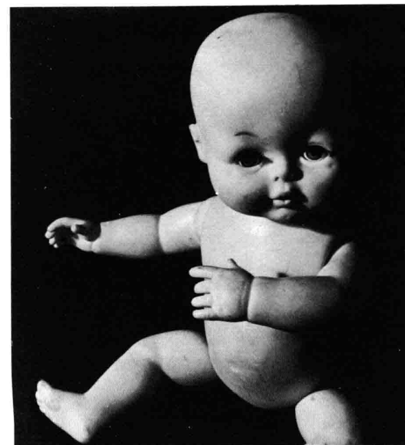
Doll rotationally cast in PVC plastisol.
