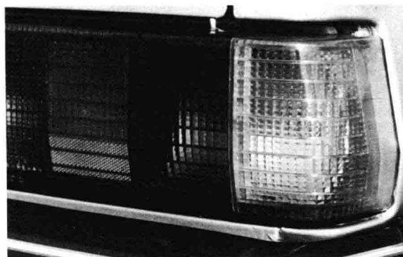
Car rear light injection moulded in acrylic.
