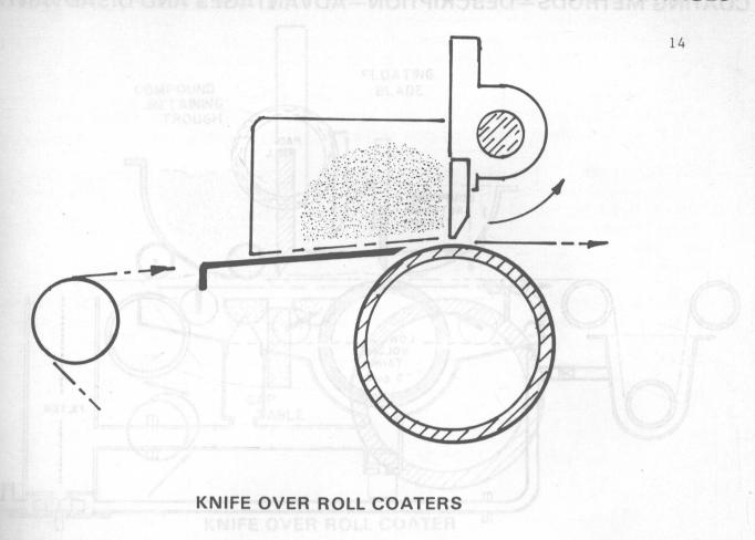
e over roll or "gap coating" applies mainly to the drapery industry. This method incorporates a precision positioned directly below a blade assembly.
