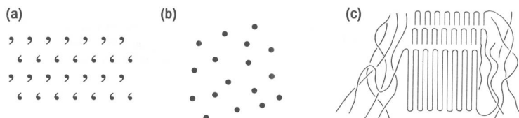
Figure 1.2. Regularity and order in matter. Some materials consist of many identical copies of one molecule, well ordered as in a crystal (a), or in random relative arrangement as in a gas or fluid (b). Other materials consist of non-identical molecules, with some domains exhibiting a high degree of local order and others disordered (c).
