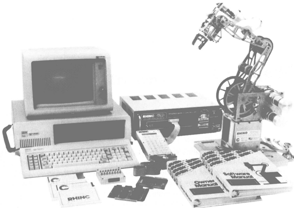
Figure 1.1: Rhino XR-3 Robotic System (Courtesy of Rhino Robots, Inc., Champaign, IL, Robotic arm developed and manufactured in the U.S.A.)
