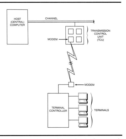
Figure 1-1 Communications Path from Central Computer
