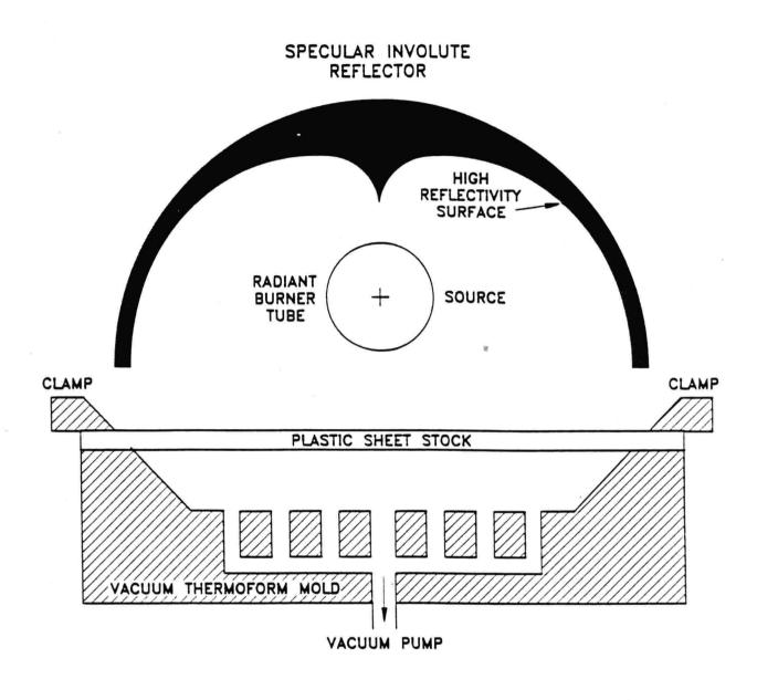
Figure 1.1. A High Efficiency Gas-Fired Proximity Heater for Vacuum Molding Thermoplastics.
