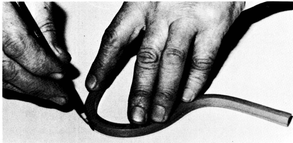
1.13 Drawing irregular curved lines. (a) French curves (Jakar) (b) Flexible curve (Jakar-flex).
