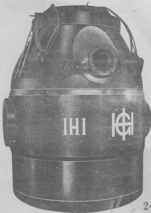
Fig. 25 Turbo Compressor 透平壓縮機 for Kawasaki Steel Corp.(1960) Type: Double suction six stages Capacity: 28,000 Nm 3 /h Max. 35,300 Nm 3 /h Pressure: 4.9 kg/cm 2 G Motor: 3,100 kW 3,000 rpm.
