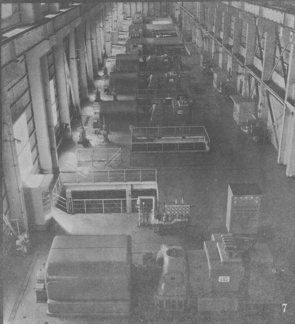
Fig. 7 軸流式鼓風機 Axial Blower (9,200kW × 1, 8,500kW × 3) for Yawata Iron & Steel Co., Ltd. (1960) Type: Multi stage Axial flow Capacity: 2,200-3,200 Nm 3 /min. Pressure: 1.0-2.1 Kg/cm 2 g Motor: 9,200kW-3,600rpm
