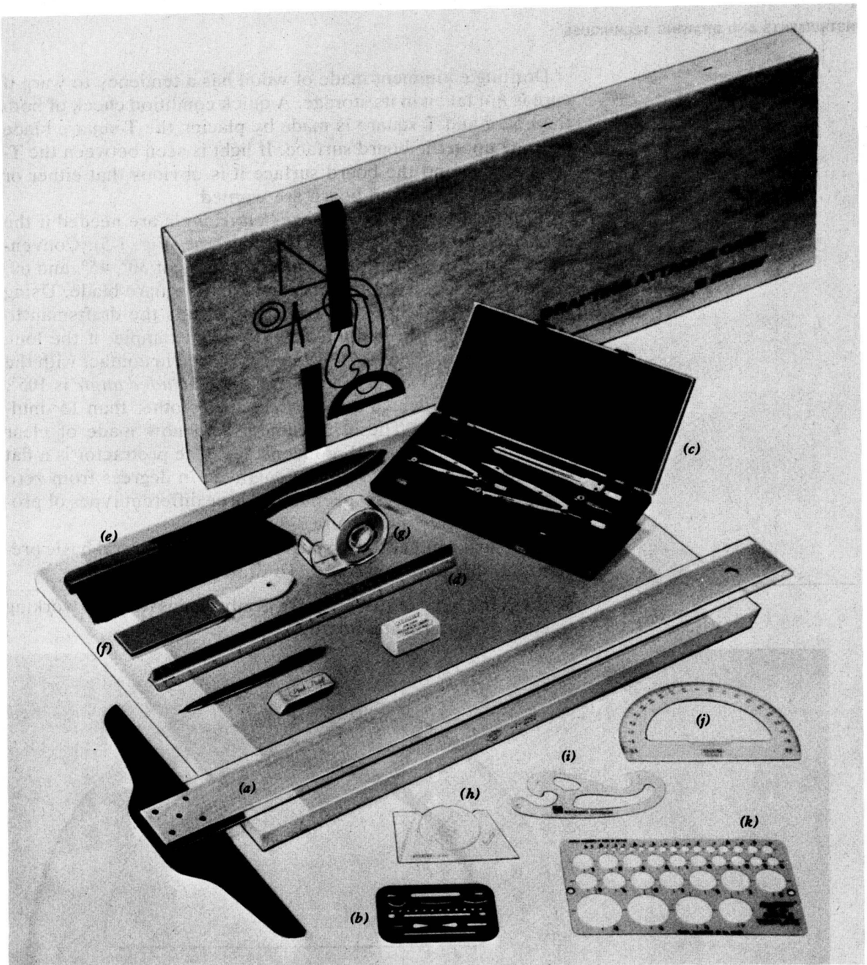
Figure 1-2 Drafting attache case. (Courtesy Bruning Div. AM.) (a) T-square; (b) erasing shield; (c) instruments case; (d) triangular scale; (e) dust brush; (f) sandpaper block; (g) cellophane tape; (h) lettering guideline template; (i) French curve; (j) protractor; (k) circle template.
