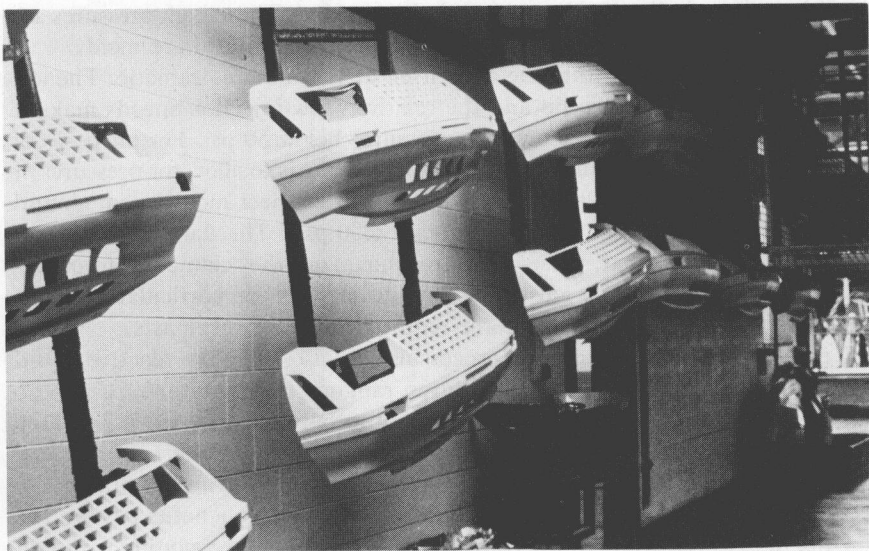
FIG. 2—Ford Mustang fascias, a good demonstration of the complex shapes possible with RIM. Photo courtesy Ford Motor Company.
