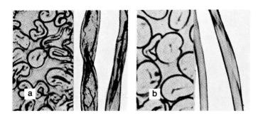
Figure 1-1 Cross-sectional and longitudinal views of cotton fibers under a microscope: (a) natural cotton fiber (Courtesy U.S. Testing Co.) and (b) mercerized cotton fiber. (Courtesy U.S. Department of Agriculture)
