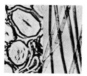
Figure 1-2 Cross-sectional and longitudinal views of linen (flax) fiber under a microscope. (Courtesy U.S. Testing Co.)
