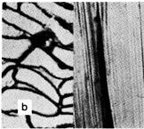
Figure 1-4 Cross-sectional and longitudinal views of silk fibers under a microscope: (a) cultivated silk fiber (Courtesy U.S. Testing Co.) and (b) wild, or tussah, silk fiber. (Courtesy U.S. Department of Agriculture)
