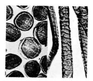
Figure 1-3 Cross-sectional and longitudinal views of wool fiber under a microscope. (Courtesy American Woolen Co.)
