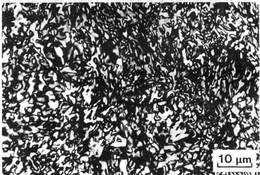
Figure 4. Optical micrograph of a coke surface showing an optical texture of medium- and coarse-grained mosaics, 1.5 - 10\text{ }\mu\text{m} diameter, OTI = 5.
